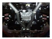
6. When you have everything in place, firmly tighten all bolts and clamps down securely. Inspect all fasteners after 25-50 miles of operation and retighten as necessary.
